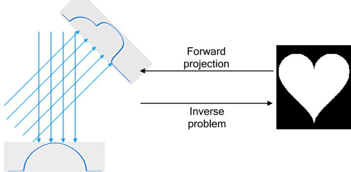
**Contribution:** We propose a direct segmentation method from projection data. Its main benefit is to directly optimize the error between sinogram data and the segmentation. The segmentation is represented by a parametric curve, which can reduce the pixel artifacts and provide more accurate geometrical measurements than traditional methods.
