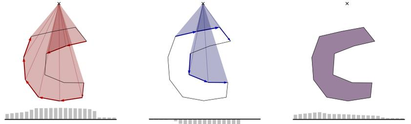
Illustration of forward model with fan beam, given a projection angle  $\theta$
