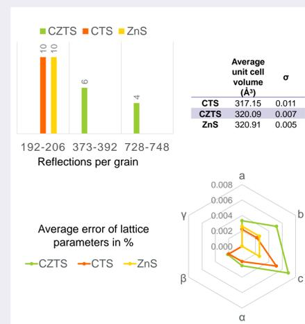
Top: GrainSpotter identified 30 grains fitted to CZTS. Completeness of the grains (observed/expected reflections) for ZnS and 60% of CZTS is above 90%, whereas for CTS is around 25%. The volume of each phase corresponds to the unit cell of the phases. Bottom right: Average error among lattice parameters of the unit cells of the identified grains.
