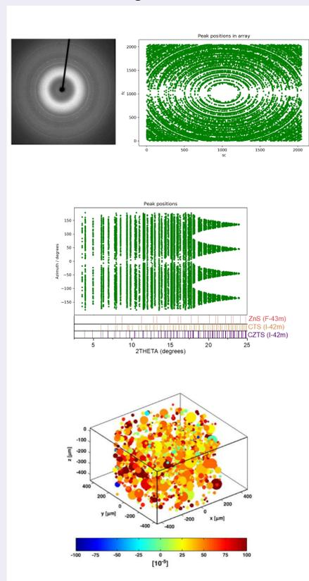
Top left: Diffraction pattern showing powder rings with spots known as reflections. Top right: Filtered reflections of the full set of diffraction images. Middle: Azimuthal projection of the diffraction spots and the position of the reflections of the unit cells. Bottom: 3D map of the position, volume (given by size of the sphere) and axial strain of 1118 grains of Cu. (Oddershede et al. 2011)
