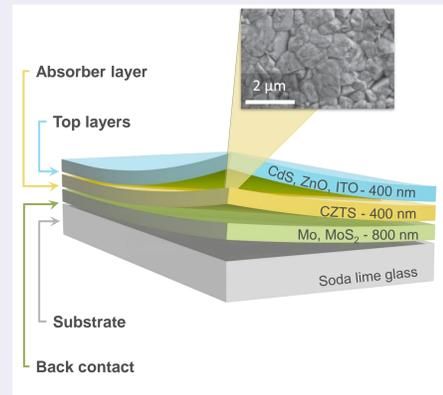
The material. The absorber layer of kesterite solar cells is composed of CZTS and secondary phases: ZnS and  $\text{Cu}_2\text{SnS}_3$ ,  $\text{Cu}_2\text{S}$ ,  $\text{SnS}_2$ .
