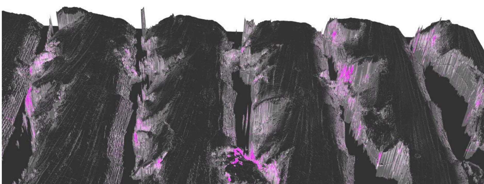
Figure 3: 3D visualization of engineered surface geometry based on data from a scanning electron microscope (SEM)
